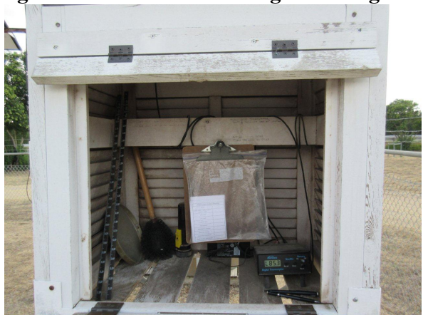
Figure 4-6. Thermometer housing Box
