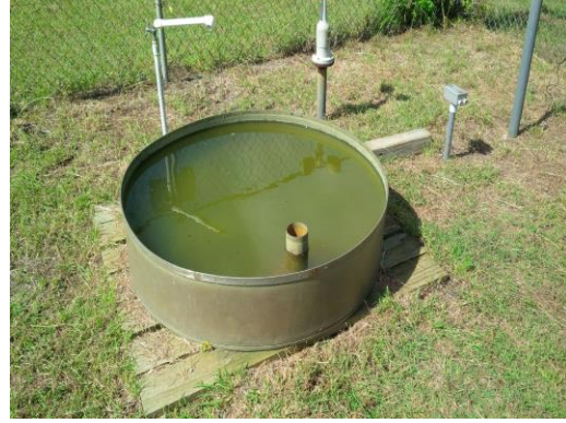
Figure 4-1. Evaporation Pan at Stillhouse Hollow Lake
