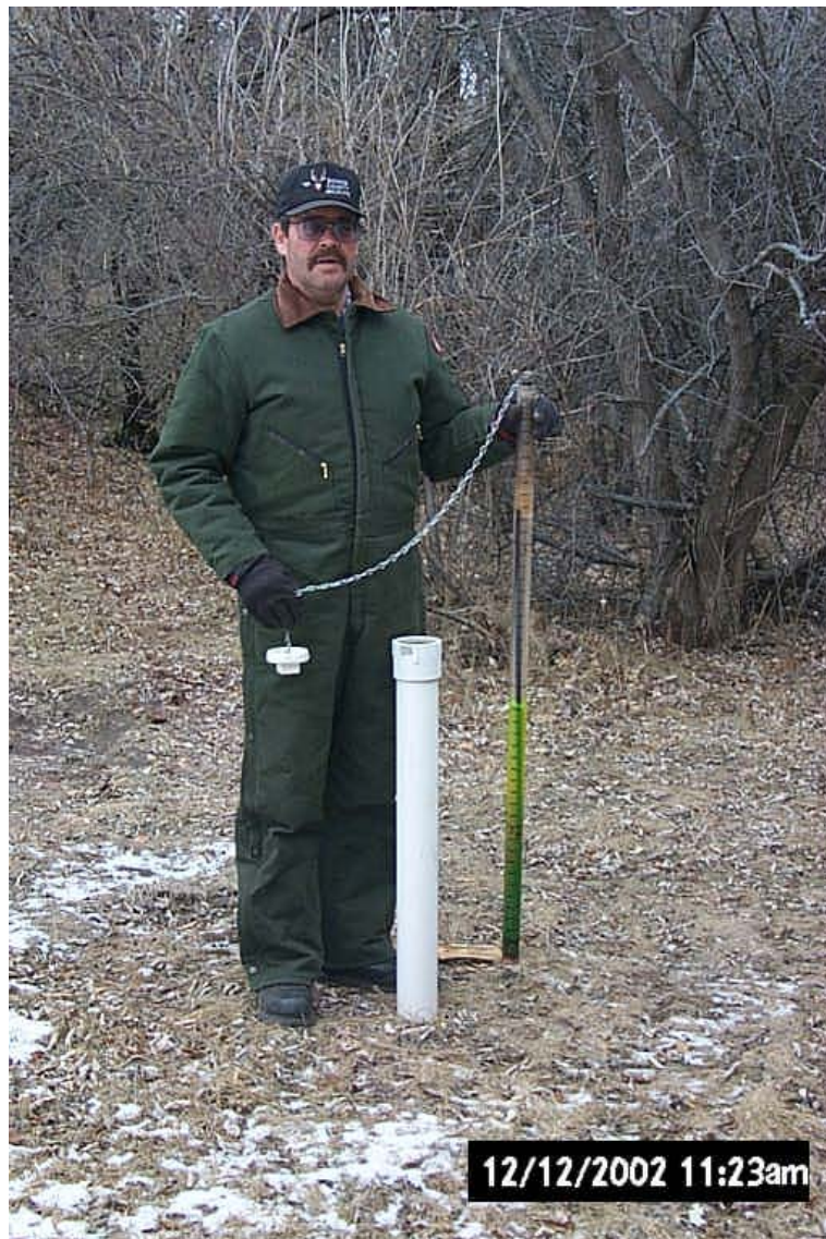
Figure 5-9. “Goose” with Frost Tube in Need of Repair.
